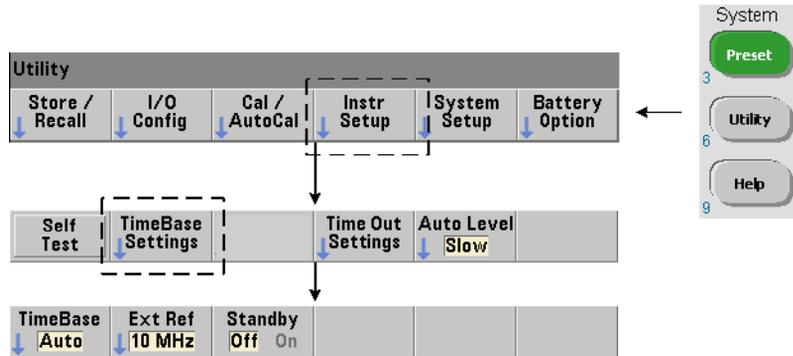
53210A measurements are based on a reference oscillator - also referred to as an internal/external clock or time base. A valid reference oscillator signal must be present for measurements to occur.
