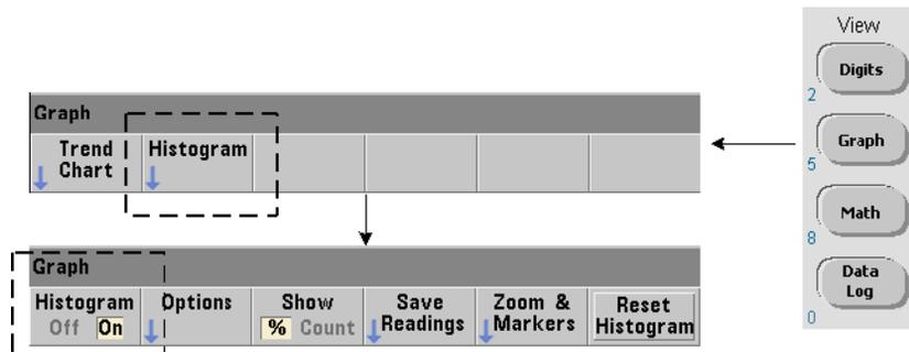
At power-on or when the front panel **Preset** key is pressed, numeric data is displayed. Remotely, histograms can be displayed by changing the display mode using the command:
