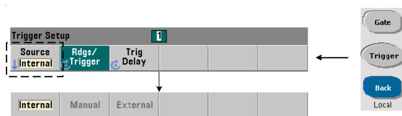
The system trigger is configured using the commands within the **TRIGger** and **SAMPle** subsystems. Figure 5-2 show the sequence in which the commands are commonly used.
