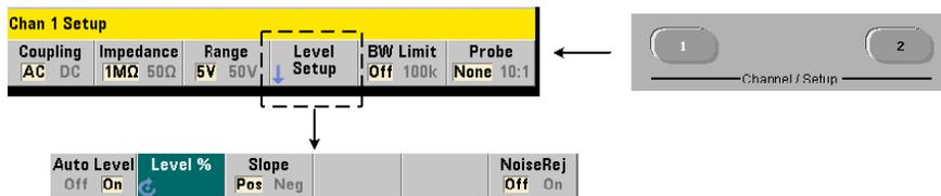
The threshold level is the trigger (input) level at which the counter begins the signal count (i.e. measurement). This level is the center of the hysteresis band - the band which represents counter sensitivity. For a count to occur, the signal must cross the upper and lower limits of the band in opposite directions (polarities). Figure 4-4 identifies these characteristics and conditions of the input signal. The dynamic range of the input signal is indicated on the front panel.
