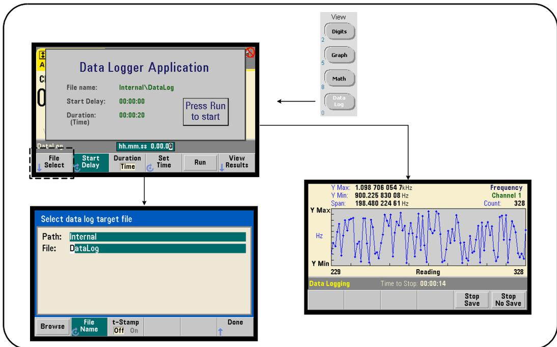
Figure 6-11 Starting the Counter Data Logger.
