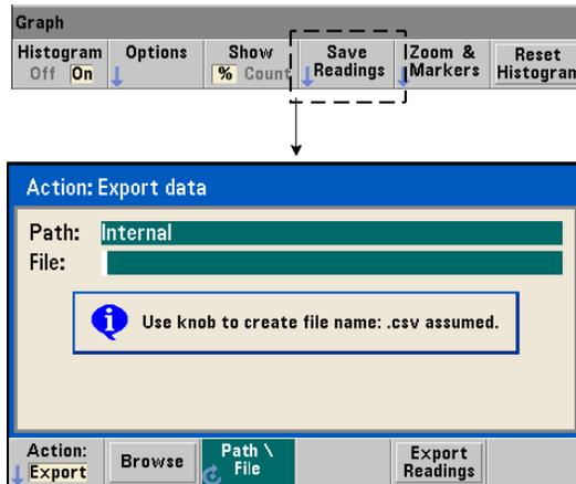
The readings used to create the histogram can be saved to internal flash memory or to an external USB memory device as comma-separated values (CSV) in one measurement per line ASCII format.
