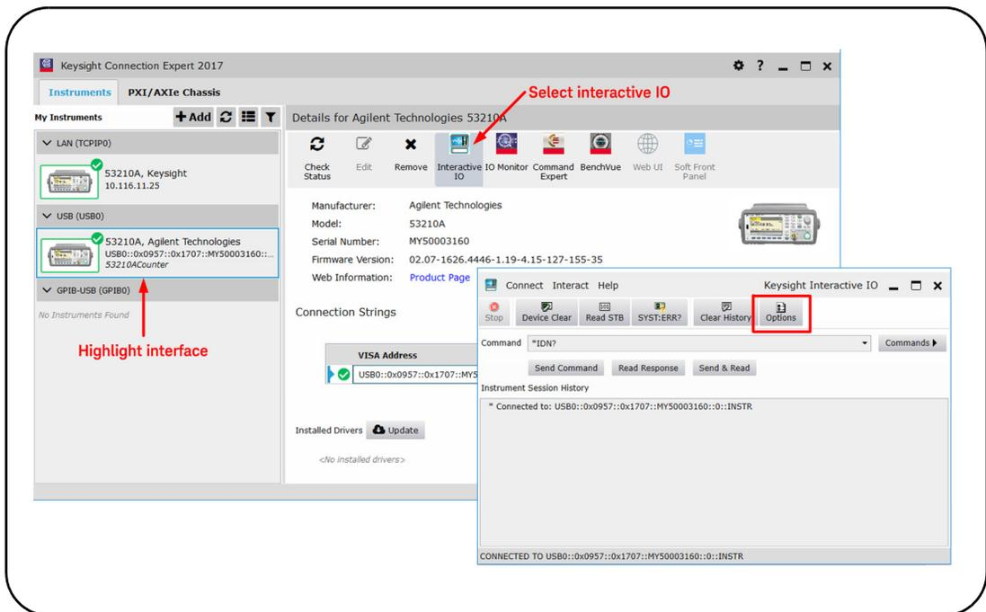
**Figure 2-8** Starting Interactive IO for a Selected Interface.
