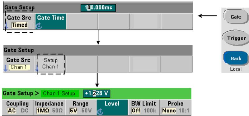
For external source `INPut[1]`, a **fixed** input threshold voltage must be specified in addition to the gate signal polarity. This is done using the command:
