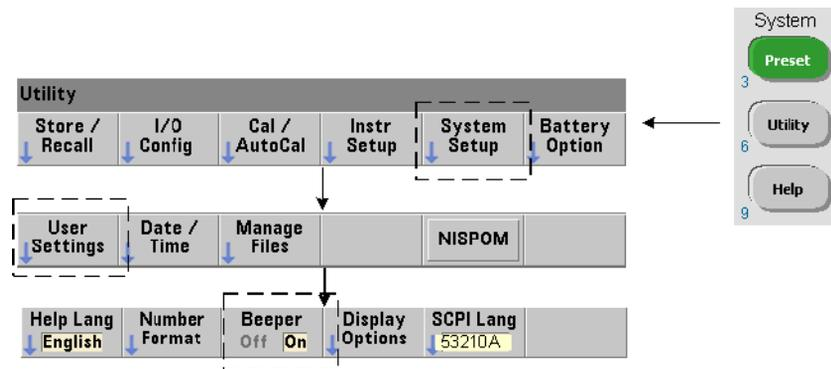
The counter's Beeper is an indication of a programming error generated from the front panel or over the remote interface. Turning off the beeper disables the audio indication.
