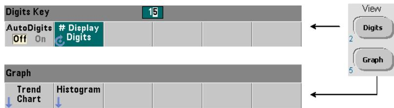
With **AutoDigits On**, the number of digits displayed is automatically set based on the gate time. When **Off**, the number of digits is set with the rotary knob or **[Shift]**ed numeric keys. See "[Resolution and Gate Time](#)" in [Chapter 5](#) for more information when **AutoDigits On** is set.
