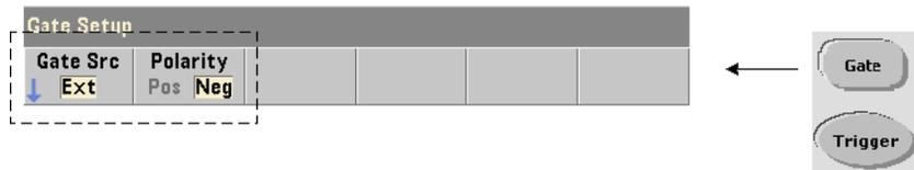
When using any external gate source the polarity of the gate signal and therefore, the duration of the gate, is set or changed with the command:
