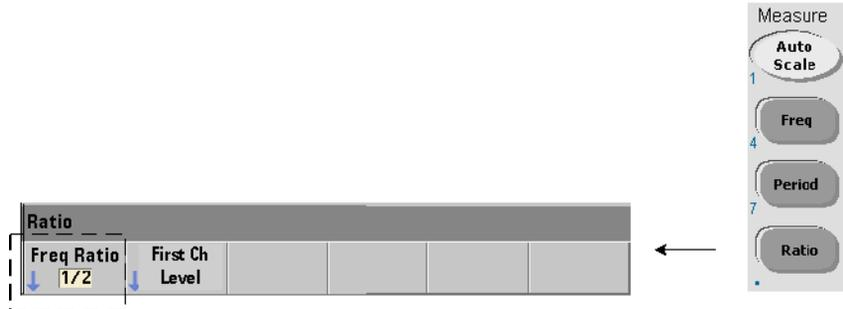
A frequency ratio measurement is the measurement of two signals in which one signal generally serves as a reference (Figure 3-2). The signals can be different wave shapes and applied to any 2-channel combination on the counter.
