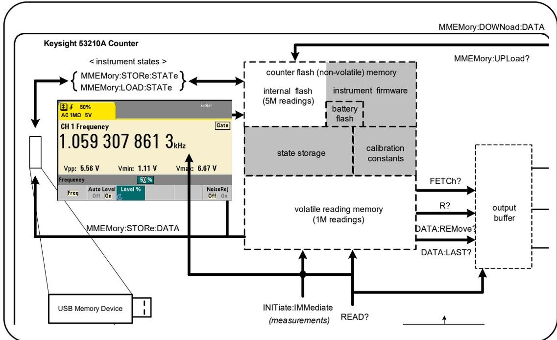
**Figure 7-1** Data Flow within the 53210A Counter.
