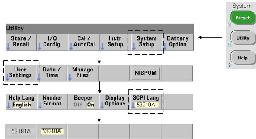
If the 53210A is sometimes used in 53181A SCPI language (emulation) mode, the instrument must be returned to its original (53210A) mode before the firmware can be updated.
