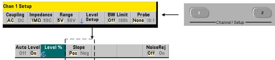
The slope (edge) of the input signal on which the threshold level occurs is specified with the command:
