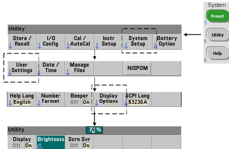
Note that pressing any key with the display turned off, turns the display back on.
