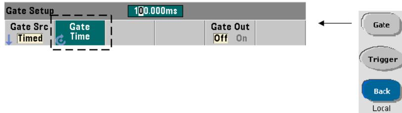
A measurement gate time can be specified directly with the command:
