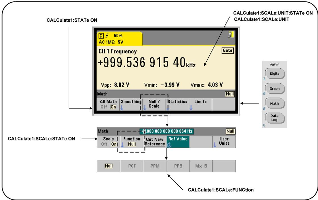
**Figure 6-2** 53210A Display with Scaling Functions Enabled.
