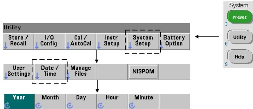
The date and time settings for the counter's real-time clock are set using the commands:
