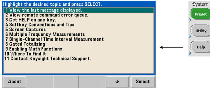
Instrument help is available by pressing and holding any front panel key or softkey. Pressing the **Help** key enables you to select additional help topics including front panel measurement examples.
