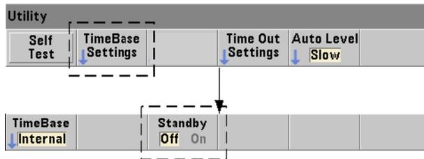
Standby power to maintain the operating temperature of the counter's internal OCXO reference oscillator (Option 010) is provided by the line voltage or from Battery Option 300. Standby power is enabled and disabled using the command:
