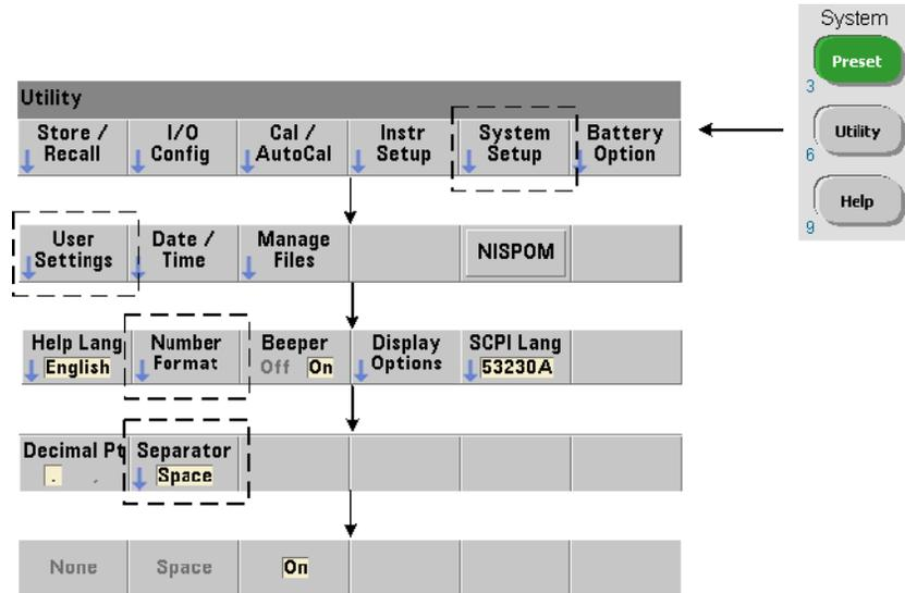
The format also applies to numeric readings within trend charts, histograms, limit testing, etc.
