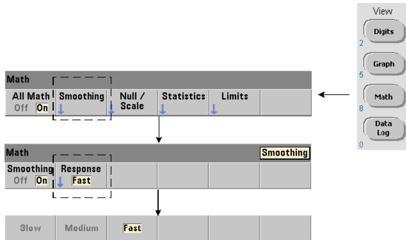
Measurements can be “smoothed” and scaled prior to performing math operations on the incoming data.
