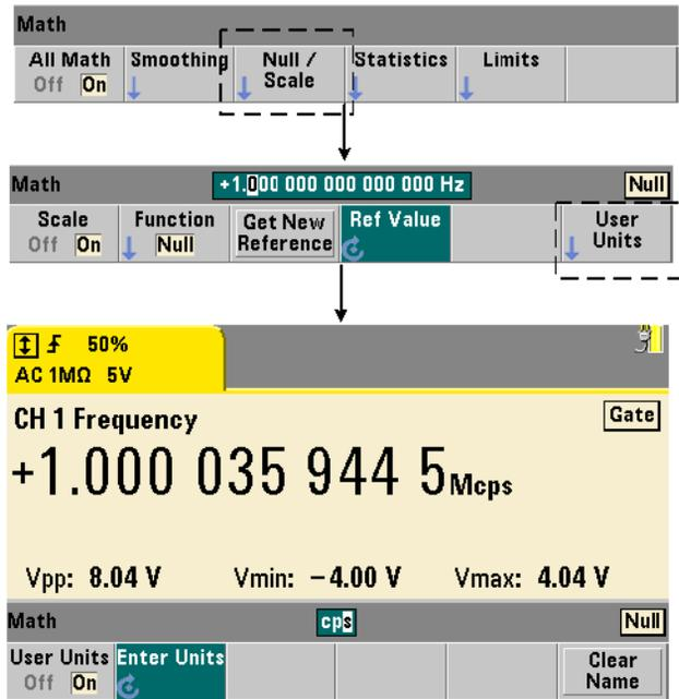
For ease in identifying readings from the front panel, a user-defined “units string” can be assigned to any scale function. The user string replaces the instrument-assigned measurement units (Hz, pct, ppm, ...). The unit prefix ( $\mu$ , m, k, M) remains.
