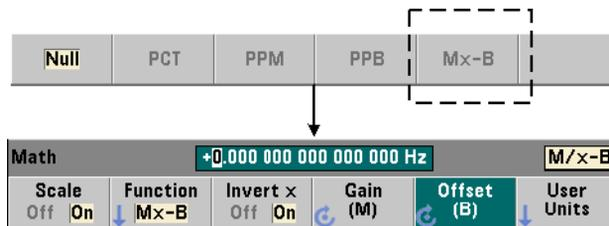
Scaling function results must be in the range of  $-1.0E+24$  to  $-1.0E-24$ ,  $0.0$ , or  $+1.0E-24$  to  $1.0E+24$ . Results outside these limits will be replaced with  $-9.9E+37$  (negative infinity),  $0$ , or  $+9.9E+37$  (positive infinity).
