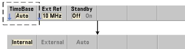
The reference oscillator (time base) is either the counter's internal oscillator or the internal oscillator tuned to an external reference. The source commands are:
