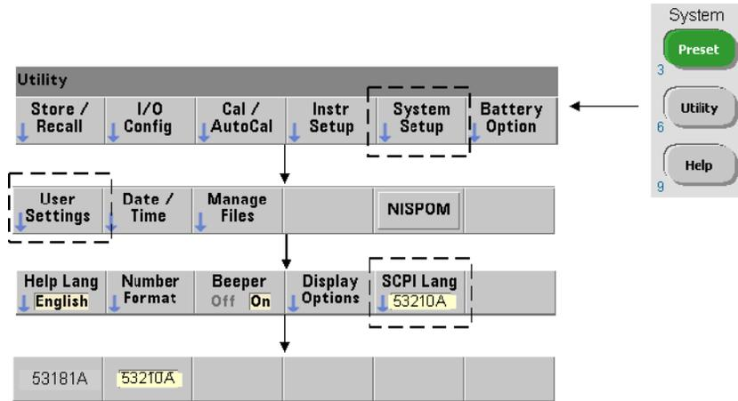
The 53210A's emulation mode enables the Keysight 53181A SCPI command set to be used with the counter.
