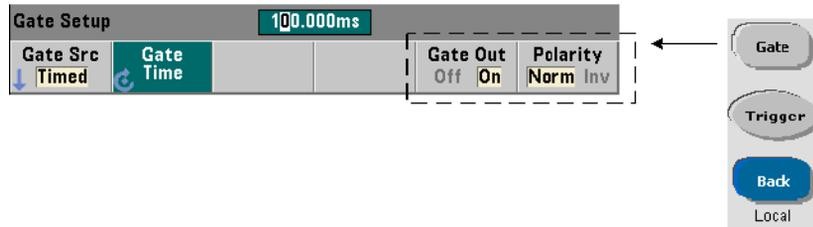
For timing and synchronization with other instruments, gate signals from source **TIME** (internal) and **INPut[1]** can be routed to the rear panel
