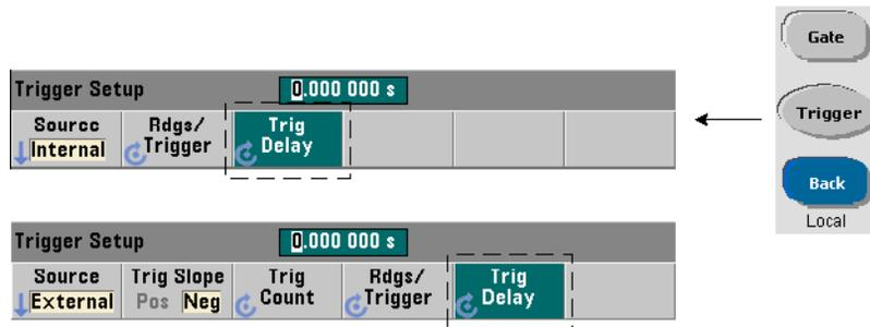
The delay between receipt of the internal or external system trigger signal and the start of the first measurement (Figure 5-2) is set with the command:
