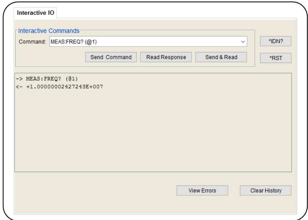
**Figure 2-2** The Web UI SCPI Command Interface.
