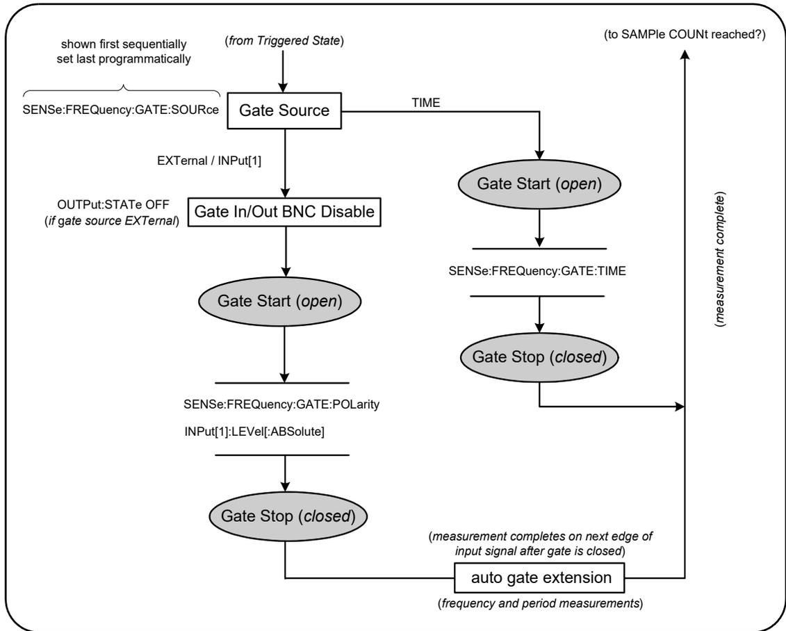
**Figure 5-3** Trigger and Gate Cycle - Gating.
