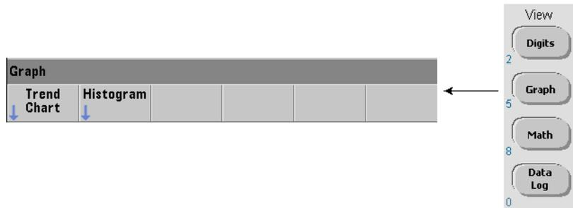
At power-on or following a reset (\*RST) or instrument preset (**Preset**), numeric data is displayed. The display can be changed to a trend chart by changing the display mode using the command:
