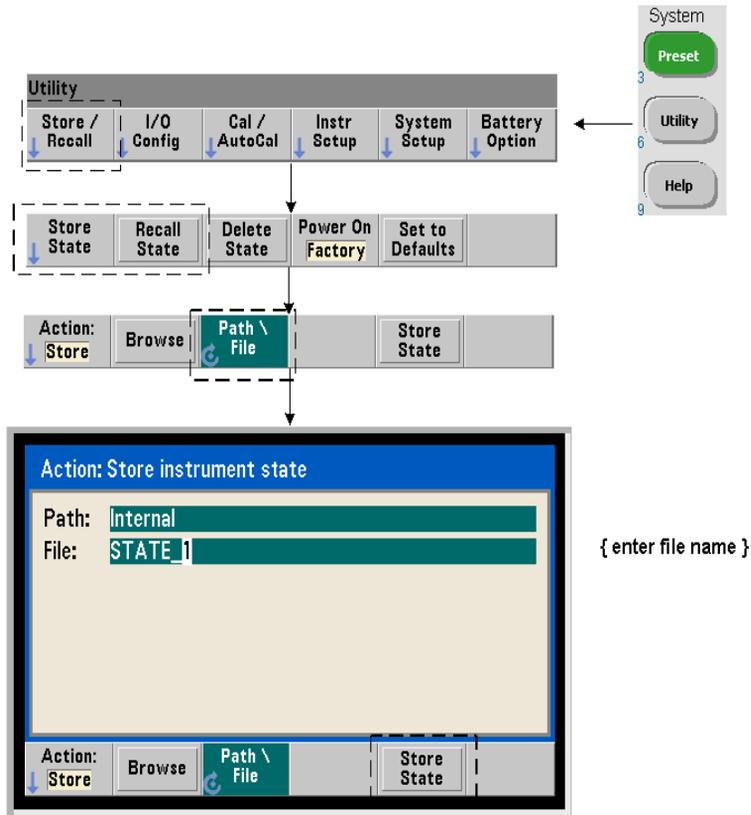
Instrument states can be stored in the instrument’s internal flash memory or on a USB memory device and recalled later to restore a specific configuration (Figure 7-2).
