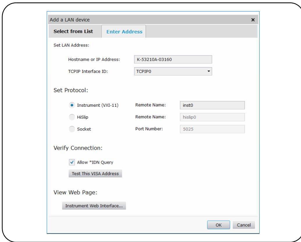
**Figure 2-5** Adding a Sockets Connection.
