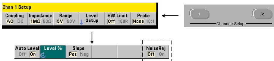
Threshold sensitivity (Figure 4-4) to the input signal is a function of the amount of noise rejection or hysteresis. Noise rejection (the hysteresis band) at the counter input is increased or decreased with the command:
