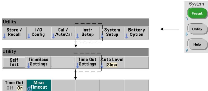
The measurement time-out is the time allowed for **each** measurement to complete. If a measurement **does not** complete before the time out expires, **9.91E37** (not a number) is returned and the display indication is: - - - - - . The sequence continues with the next reading in the sample count.
