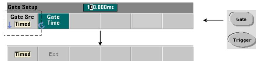
Gate sources **EXTernal1** and **INPut[1]** are external sources. **EXTernal1** is the counter's rear panel 'Gate In/Out' BNC, and **INPut[1]** is the counter's channel 1 input (front or rear panel - Opt. 201). Note that the **INPut[1]** source is only available when channel 2 is installed (Option 106 or 115) and is the measurement channel.
