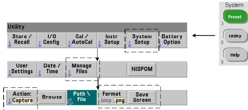
The content captured is the display state at the time the **[Utility]** key is pressed. The file format is selectable as either **bmp** (bitmap file format) or **png** (portable network graphics (bitmap) format). Files may be store in internal flash memory or to an external USB device.
