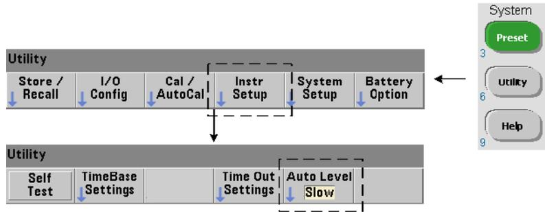
Slow sets the minimum frequency for auto-leveling at 50 Hz. Fast sets the minimum frequency for auto-leveling at 10 kHz.
