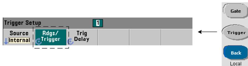
The trigger count multiplied by the sample count (**TRIG:COUN** x **SAMP:COUN**) determines the number of readings taken before the counter returns to the *idle* state. The sample count is set with the command:
