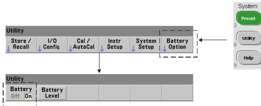
With Battery Option 300 installed and **enabled**, the 53210A counter can be operated using battery power for up to three hours.
